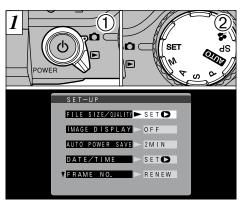
① Set the Mode switch to " ② Set the Mode dial to "SET". The SET-UP screen appears on the monitor.
